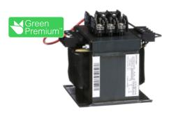
Industrial control transformer, Type TF, 1 phase, 1000VA, 240x480V primary, 120V secondary, 50/60Hz
