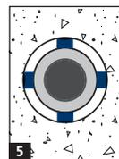
5. For proper installation, the shoulder of the setting tool must come briefly in full contact with the Smart DI+™ resulting in the blue indicator paint being removed from the raised top of the anchor. The paint will remain in the recessed portion of the top indicating full expansion.
