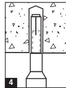
4. Once attached, insert the tip of the setting tool into the Smart DI+™ anchor and drive the internal plug fully using the rotation with hammer mode of the SDS+ drill (see table below for suggested tools).
