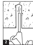
2. Blow the hole clean of dust and other materials. Insert the anchor into the hole and, if necessary, tap flush with the surface.
