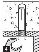
6. If using a fixture, position it, insert the bolt and tighten so as not to exceed the maximum tightening torque. Most overhead applications utilize threaded rod. Minimum thread engagement should be at least one anchor diameter.
