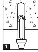
1. Drill a hole into the base material to the depth of embedment required using the appropriate Powers DI+™ Drill. The tolerances of the drill bit used must meet the requirements of ANSI Standard B212.15. Standard installation with a DI+™ Drill may result in the anchor being slightly subset from the surface. Minimum published embedment depths must be achieved by using the shoulder of the DI+™ Drill as a guide.
