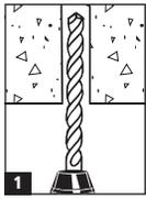
1. Drill a hole into the base material to the depth of embedment required. The tolerances of the drill bit used must meet the requirements of ANSI Standard B212.15. Use any ANSI Standard carbide drill bit.
