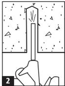
2. Blow the hole clean of dust and other materials. Insert the anchor into the hole and, if necessary tap flush with surface.
