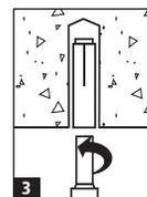
3. Slide the appropriate Powers DI+™ Tool over the DI+™ Drill used to drill the hole and twist counterclockwise to lock the setting tool onto the bit. If tool does not fit snug onto bit it may be necessary to replace the internal rubber spring plug in the tool (see ordering information). Replacement kit sold separately.
