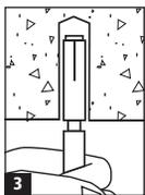
3. Using a Powers manual setting tool specifically, set the anchor by driving the tool with a sufficient number of hammer blows until the shoulder of the tool is seated against the anchor. Anchor will not hold allowable loads required if shoulder of Powers manual setting tool does not seat against anchor. Proper manual installation may not remove blue indicator paint.
