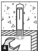
4. If using a fixture, position it, insert bolt and tighten so as not to exceed the maximum tightening torque. Most overhead applications utilize threaded rod. Minimum thread engagement should be at least one anchor diameter.
